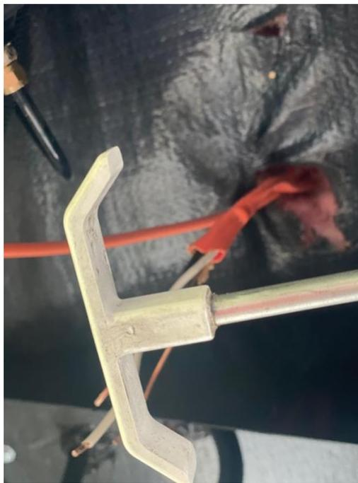
*Figure 11: New hole for inverter wires, next to freshwater tank dump handle.*
