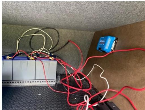
*Figure 3: Lithium completely connected with no modification to wiring length or neatness. The wiring comes through a new hole placed into the storage compartment via the front access panel of the trailer*
