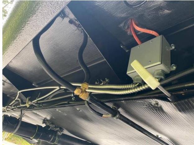
*Figure 14: Armorlite wiring to front of trailer with loops securing it to trailer frame*
