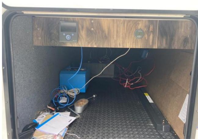
Figure 4: All components mounted to include panel placed in top space to house color controller and battery monitor
